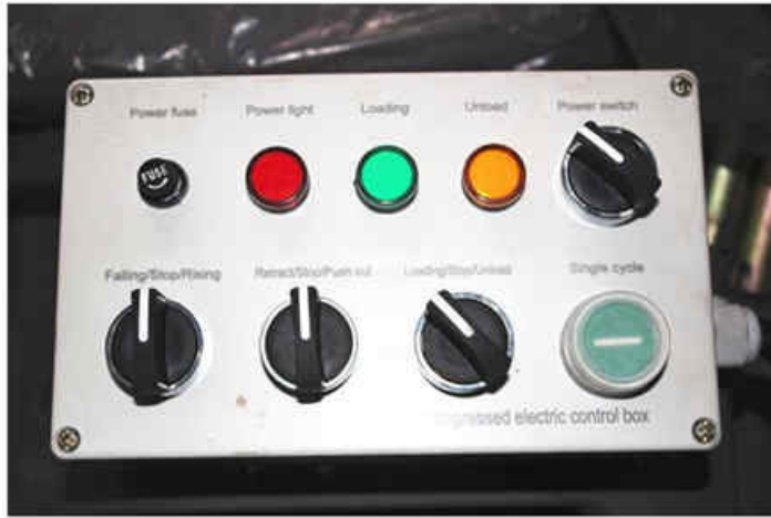
Main Control Box
